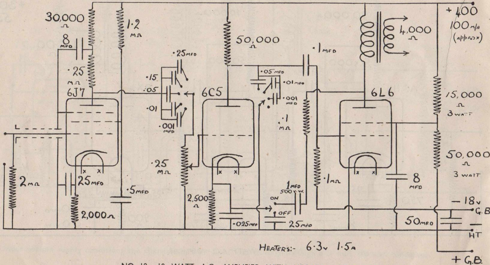
NO. 18. 10 WATT A.C. AMPLIFIER WITH NEGATIVE FEEDBACK
