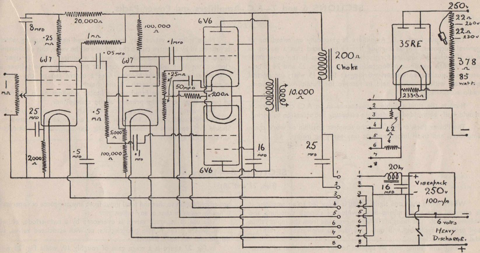
No. 16. A.C./D.C./BATTERY AMPLIFIER, 8 WATTS
