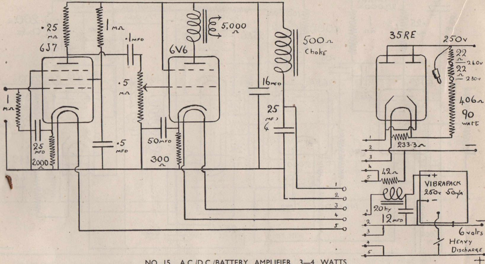
NO. 15. A.C./D.C./BATTERY AMPLIFIER, 3-4 WATTS
