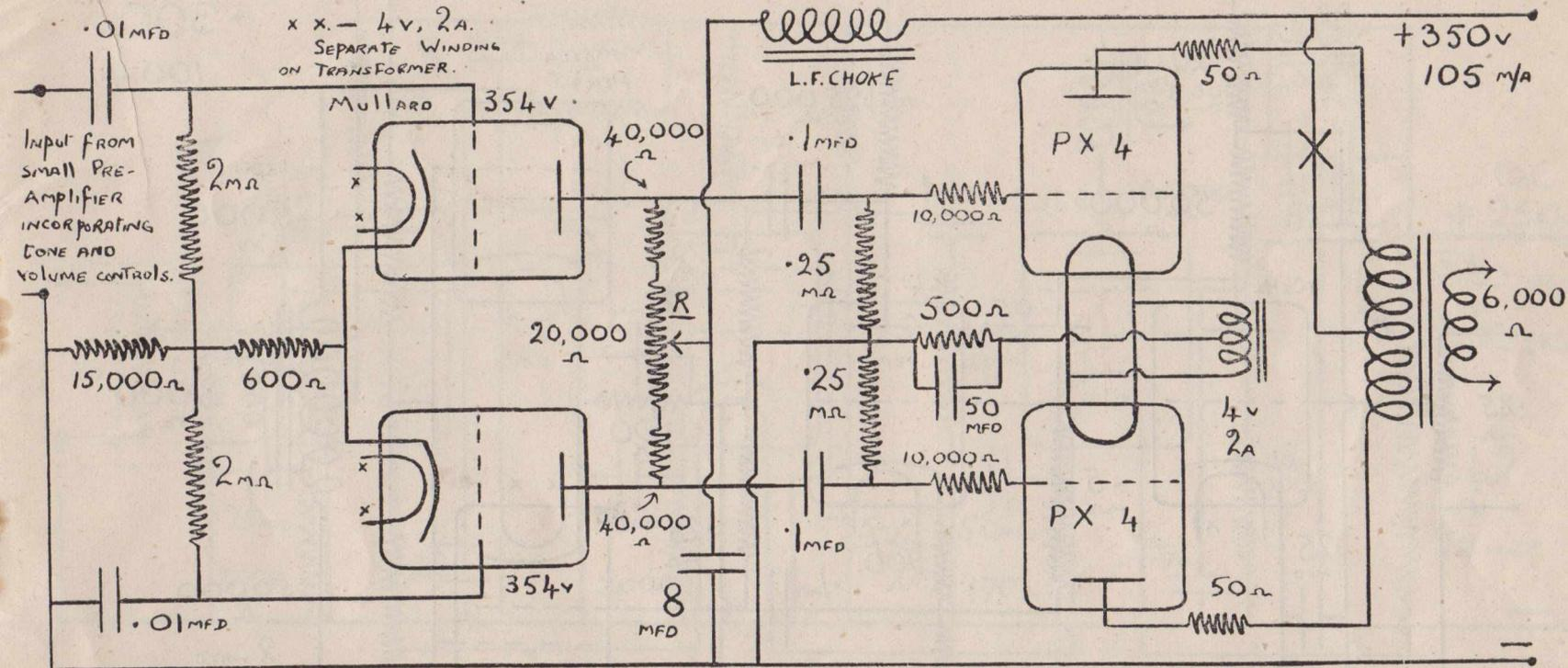
To adjust R for balance:—Insert 50  $\Omega$  resistor at X and connect phones or an oscilloscope across its ends. Feed in a small signal of constant pitch between 400—1,000 c.p.s. Adjust R until the response at X is at its *minimum*.
