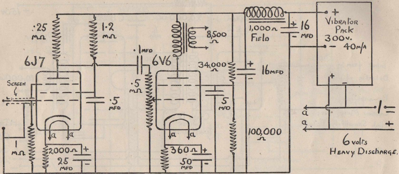
NO. 4. 4 WATT BATTERY (VIBRATOR) AMPLIFIER
